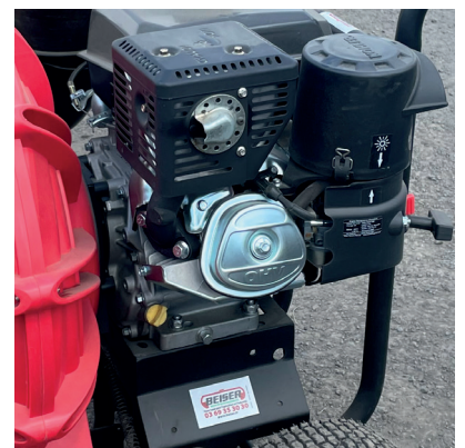
KOHLER-Motor CH440 14HP/10,5KW 4-Takt
